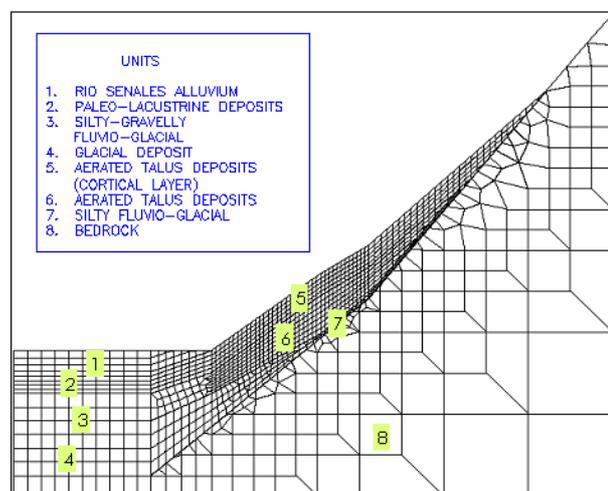
Fig. 5 – Southern slope in proximity of the operation shaft – Finite elements model mesh
