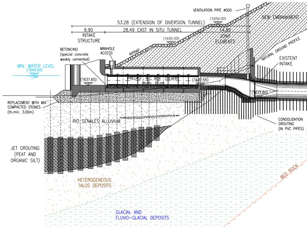
Fig. 7 – Half bottom outlet-diversion tunnel – Longitudinal profile
