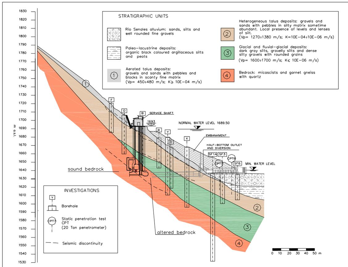
Fig. 2 – Geological section of the slope corresponding with the operation shaft area
