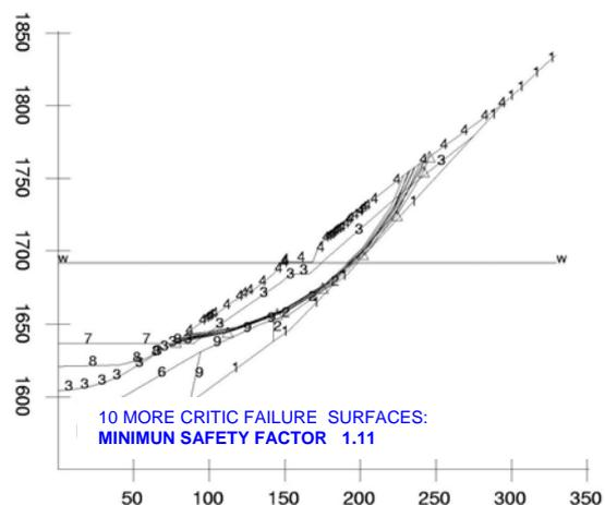
Fig. 4 – Southern slope close to the operation shaft - Stability in maximum water level conditions
