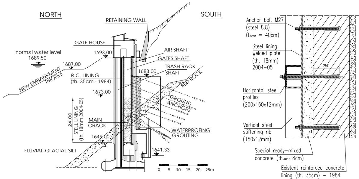
Fig. 9 – Operation shaft – Vertical section and steel lining detail
