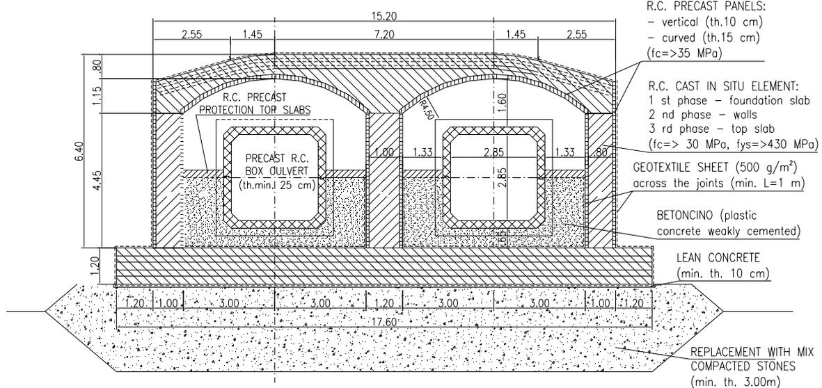
Fig. 6 – Double tunnel – Typical cross section
